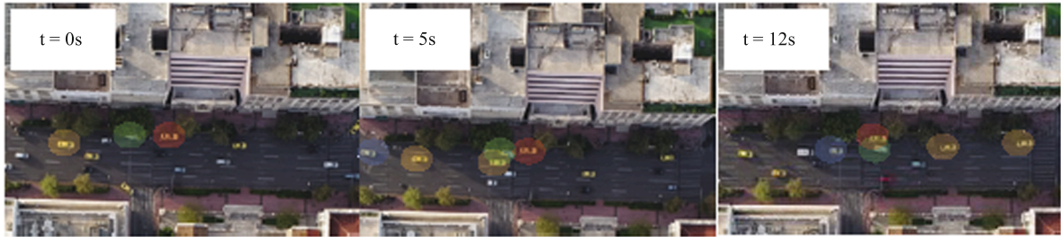
Fig. 17. The effect of a taxi (red oval) that stopped to pick-up a passenger. (For interpretation of the references to color in this figure legend, the reader is referred to the web version of this article.)
