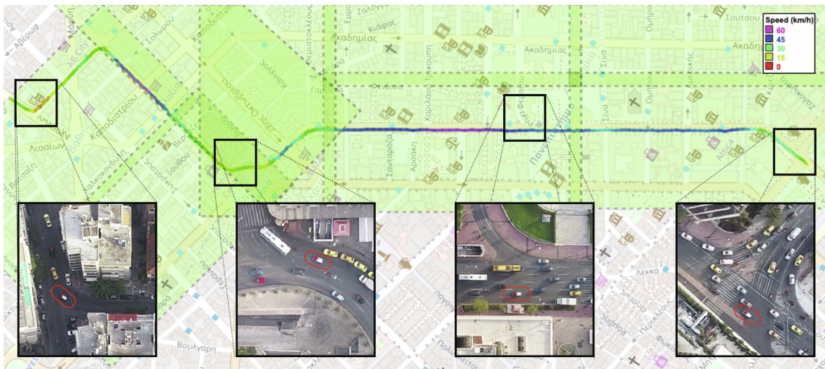
Fig. 7. The trajectory of a vehicle tracked continuously by different drones throughout the study area.
